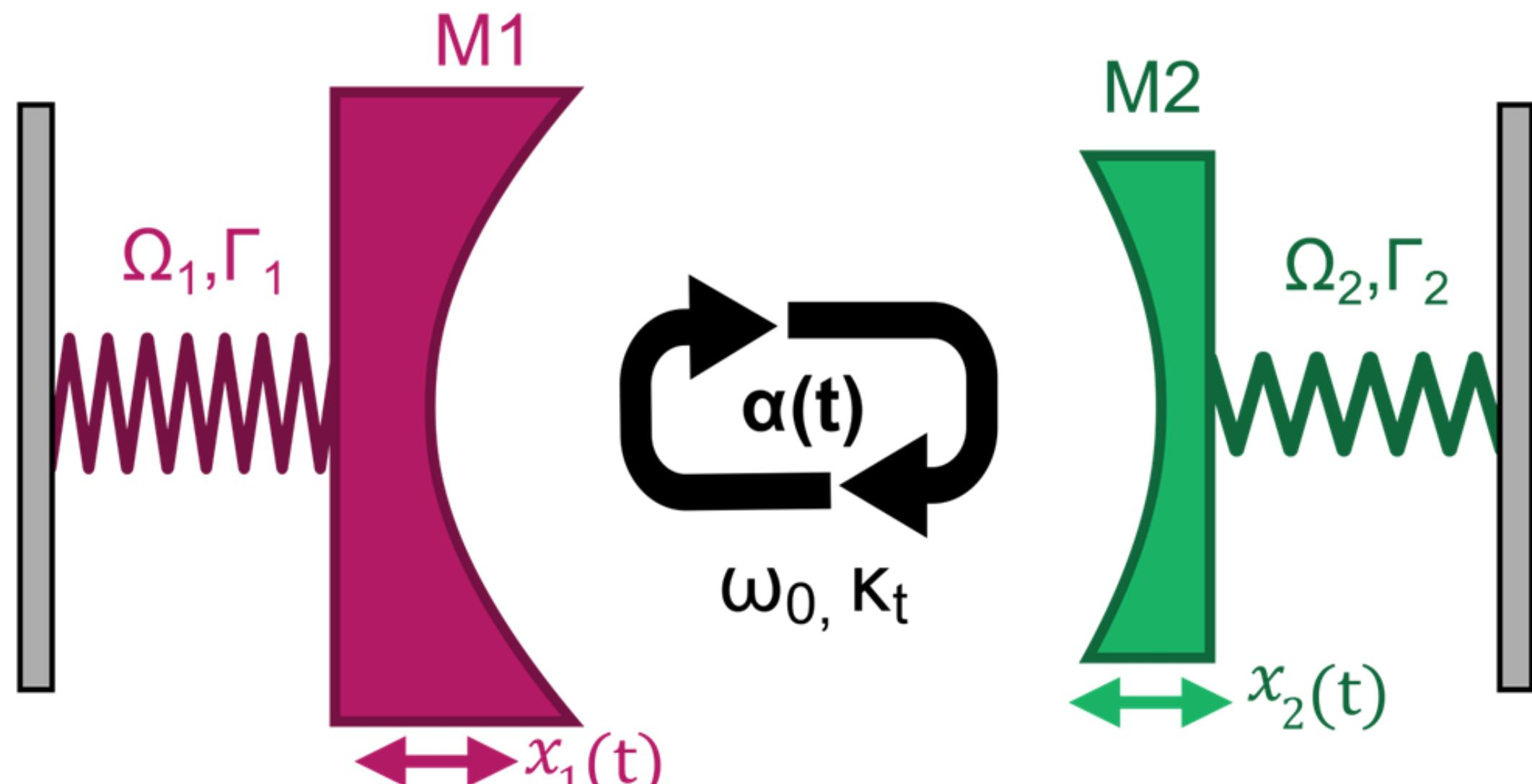
Multimode optomechanical system with **two independent mechanical modes** that interact with the same optical cavity
